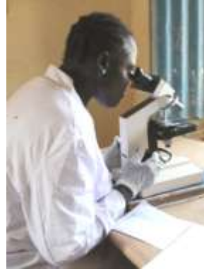
Diagnostic laboratory, microscope powered by sunlight & a mirror
